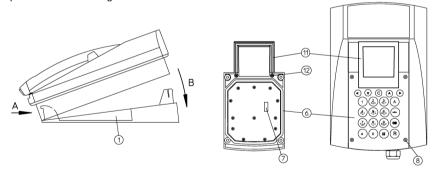
The standard handset accommodation (for the wall version) (9) can be replaced for the table version
